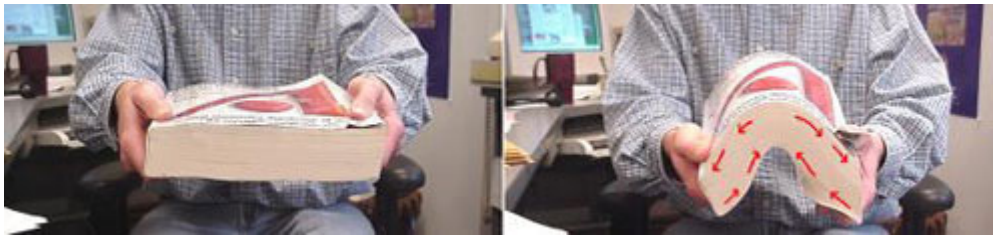
Figure 1. A demonstration using a phone book illustrates tensile and compressive stresses due to bending; the top pages stretch apart (tension) and the bottom pages push together (compression).
